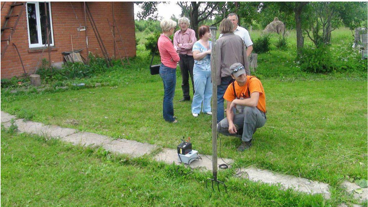
Figure 2. Measurements of soil trembling from quarry explosion at steading N1
